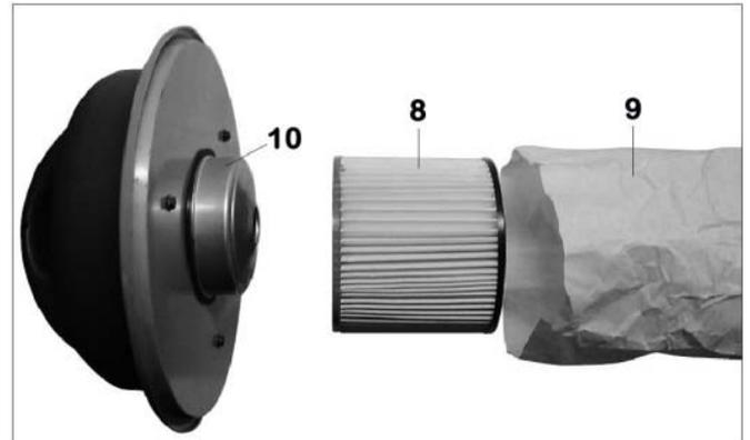
– Fold any excess bag (9) inside the filter cartridge (8).
