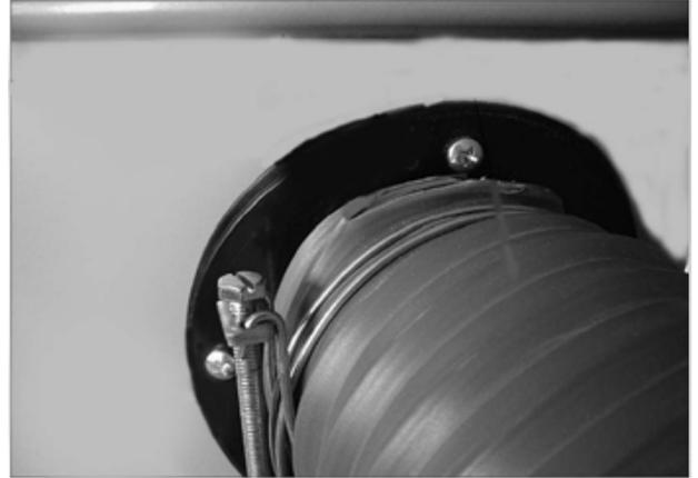
– Attach the other end of the collector hose (5) to the hose coupling (7) using the other hose clamp (6).
