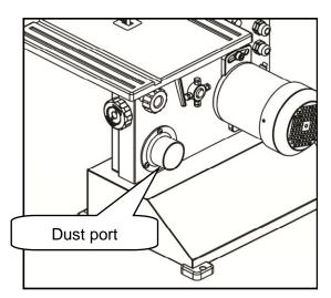
If you do not have dedicated band saw extraction, there is another chance to get rid of the saw dust. Most of debris except usual dust drifts would fall through a grating into the dust drawer. It can be easily pulled out and cleaned.
