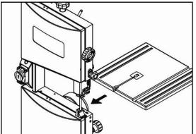
Fit the pins on the frame into the slots of the saw table bracket.
