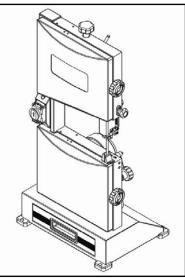
Fix the lifting handle onto top of band saw.
