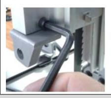
4. Loosen the screw, and remove connecting block
