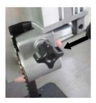
3. Loosen the socket head screw.
