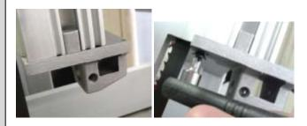
6. Tighten the socket head screw.
