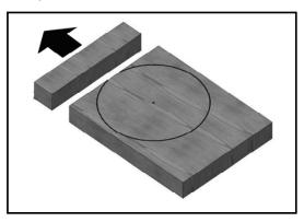
3. Put the remained workpiece with circle mark onto the table. Align the point of tangency to saw blade teeth. Set the centre pin inline to the circle centre, fix these with tightening the knob A. Turn on the band saw, slowly rotate and feed the workpiece to saw blade.
