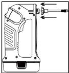
2. Push "Flexible air hose" in and turn clockwise until locked in place.
