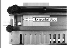
Offset the vertical stop 1/2" to the right of the horizontal stop. Ensure the vertical stop is square to the top of the jig.
