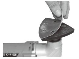
3. To remove the sanding sheet, hold it at one of the points and pull it from the sanding pad.
