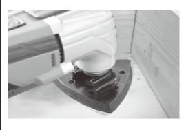
4.If sanding into comers, use the tip or corner of the sanding pad.
