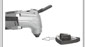
2. Fit the sanding sheet to the sanding pad.Make sure that the holes in the sanding sheet align with the holes in the sanding pad.
