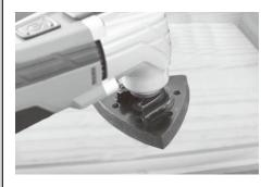
3.Let the tool to do the work and do not apply excessive pressure to the sanding pad.
