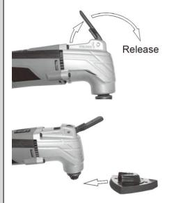
3. Move the quick release handle all the way back to lock the accessory in position.
