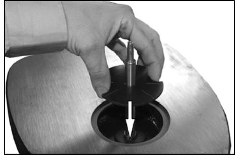
2. Slide the bobbin on to the spindle.
