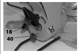
Hold the tool arm in this position and retighten the bevel lock (18).
