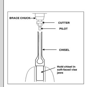
3. Use a small, triangular, smooth file to relieve the inner corners of the chisel. See Figure. Remove any burrs from the outside of the chisel with a fine oilstone.
