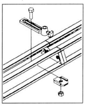
Next insert the tool rest into the holder and secure with the locking handle.
