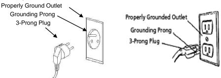
**WARNING:** Improper connection of equipment grounding conductor can result in the risk of electrical shock. equipment should be grounded while in use to protect operator from electrical shock.
